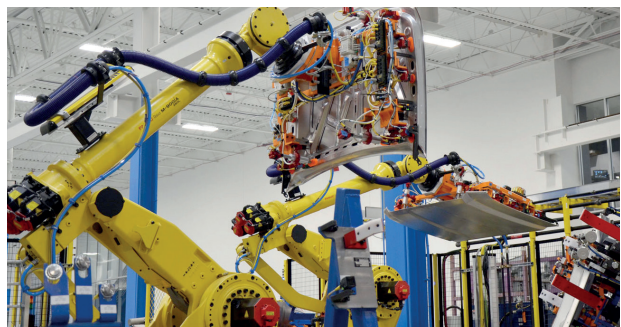
Automated production line for car body assembly
